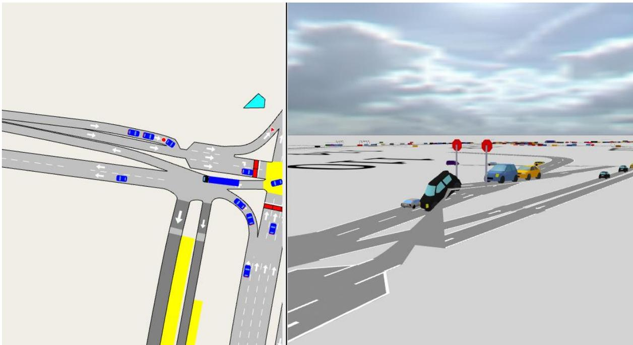
**Figure 3-1 Mismatch of Section Altitudes at Node 2801**
